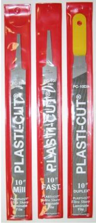
**PLASTI-CUT DUPLEX® FILES** These combine the best features of all laminate files into one versatile tool. **FAST®** cut one side, **MILL** cut other side to meet any filing situation. Wide body with straight sides gives about 10% more filing area and is best for filing into corners. One edge has no teeth for safe corner filing. The rounded tang design is safer to use and it eliminates the need for a separate handle.
